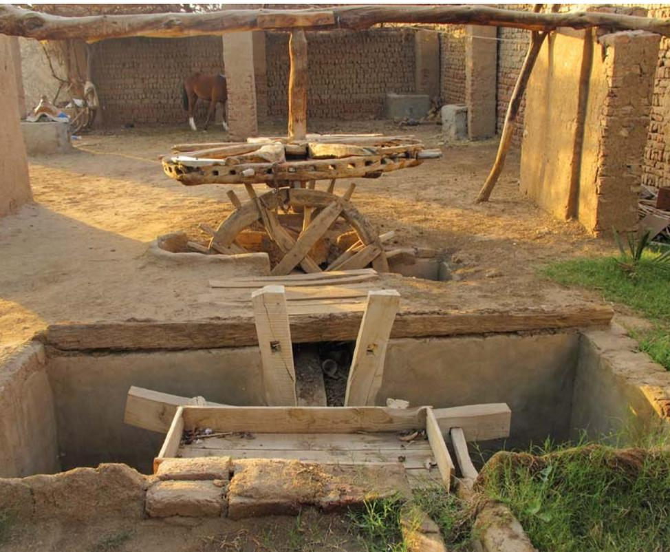
Belzoni's original assignment in Egypt was to design an irrigation tool that would prove more efficient than the traditional animal-drawn *saqiya* (waterwheel), shown here in a display near Luxor. Although his prototype appeared promising, mishap and suspicion kept it from production.
